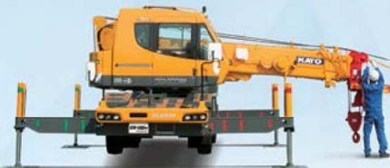
Lower the boom and attach the tension rods.
