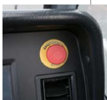
▲ Emergency engine stop switch (for crane operation)
